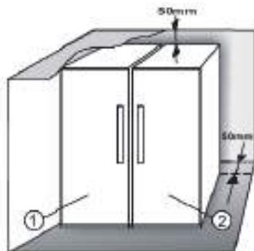
We recommended installing two appliances together using the linking-kit ③ (as shown on the drawing). You can buy it in Service.
