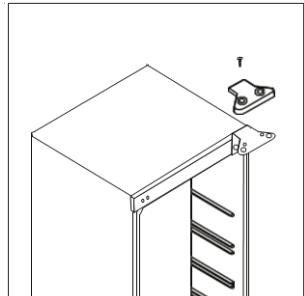
2. Open the door and unscrew the top hinge. Then lift the door to remove it from the appliance and put it on foam to avoid scratching and damaging it.
