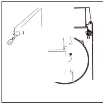
Warning! If there is a screw in the front left corner, remove it before fitting the hinge
