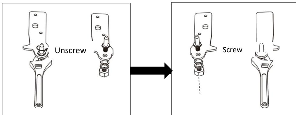
6. Install the hinge on the left side and the base of the foot on the right side. Then unscrew the two levelling feet with their original parts.
