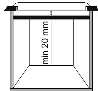
When installing an oven under the hob, separator must not be put and the minimum distance between the bottom part of the hob and the oven must not be lower than 10 mm. Do not install not cooled oven under this hob and install the oven following its own installation requirements.
