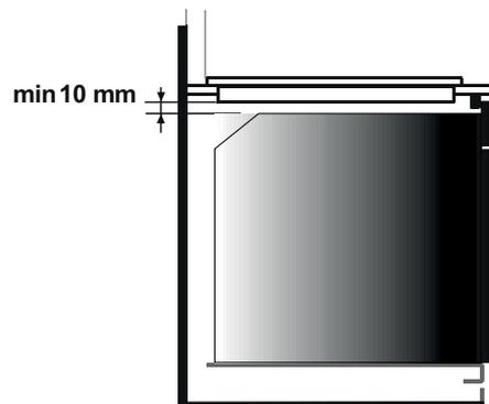
A watertight seal gasket is supplied with the hob. Fit the seal gasket around the bottom hob as described and make sure that it is properly fitted to avoid any leakage into the supporting furniture.
