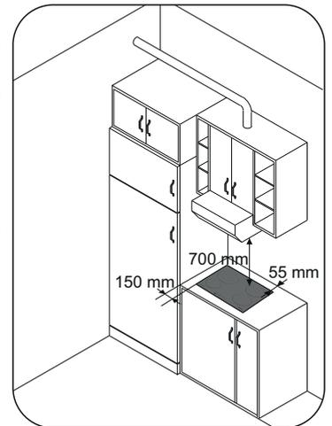
If the bottom part of the hob is adjacent to an area normally accessible for handling or cleaning operations, a separator it must be put 20 mm below the bottom part of the hob.
