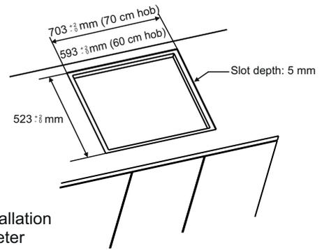
**Note:** Inner perimeter dimensions are same with standard installation
